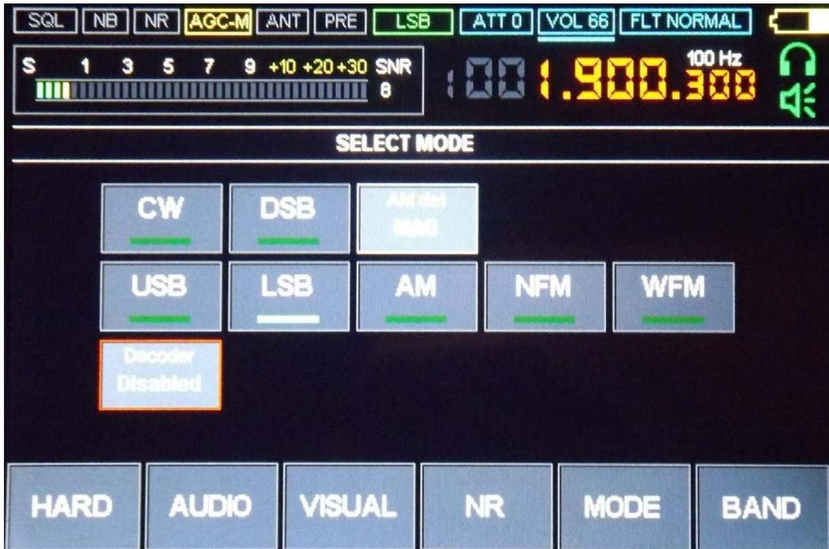
The menu is designed to select the type of modulation and control decoders. The exit is carried out by pressing the MODE button, or by pressing the encoder button ENC\_FREQ.
