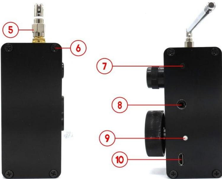
**5** Antenna socket and antenna
