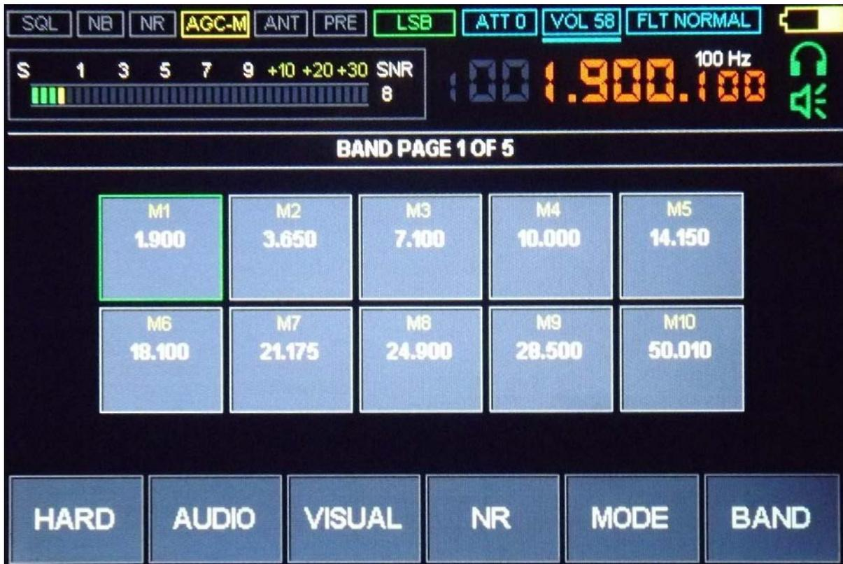
This menu is used to save and restore currently tuned frequency, modulation, and other settings to memory cells. Moving through the cells is carried out by using the encoder ENC\_FREQ. The exit is carried out by pressing the BAND button, or by pressing the encoder button ENC\_FREQ.
