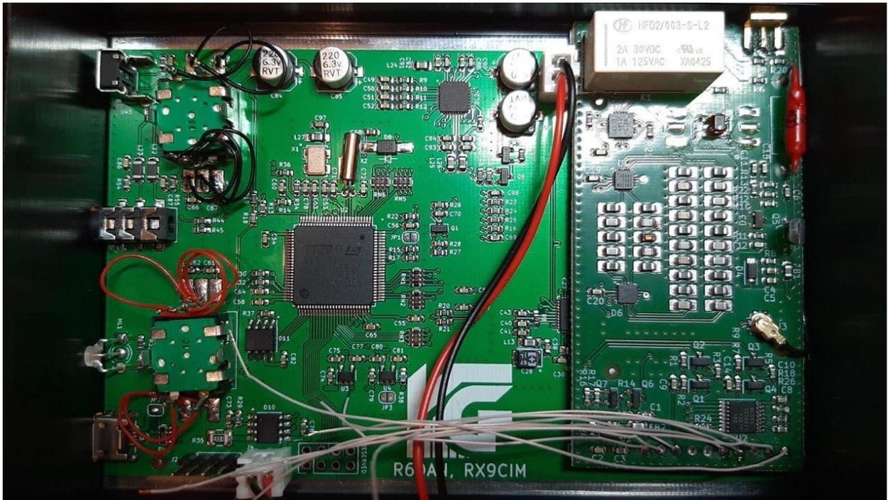
To provide an additional board with power, it is possible to connect both to the battery and to other points. For example, to the capacitor C76, located near the battery connector. The top of C76 is GND, the bottom is "+".
