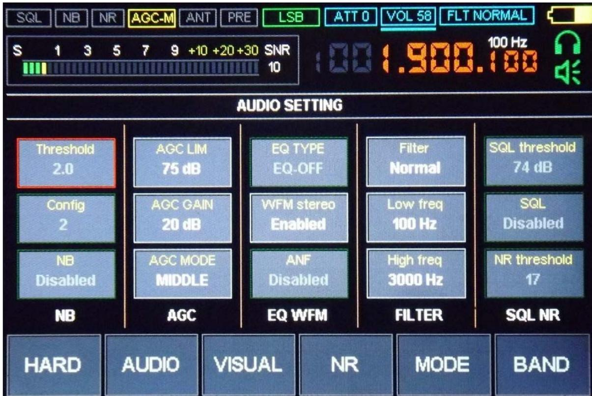
The menu is intended for selecting digital signal processing settings, mainly in the audio processing path. Exit from the menu to the main screen of work is carried out by pressing the AUDIO button, or by pressing the encoder button ENC\_FREQ.
