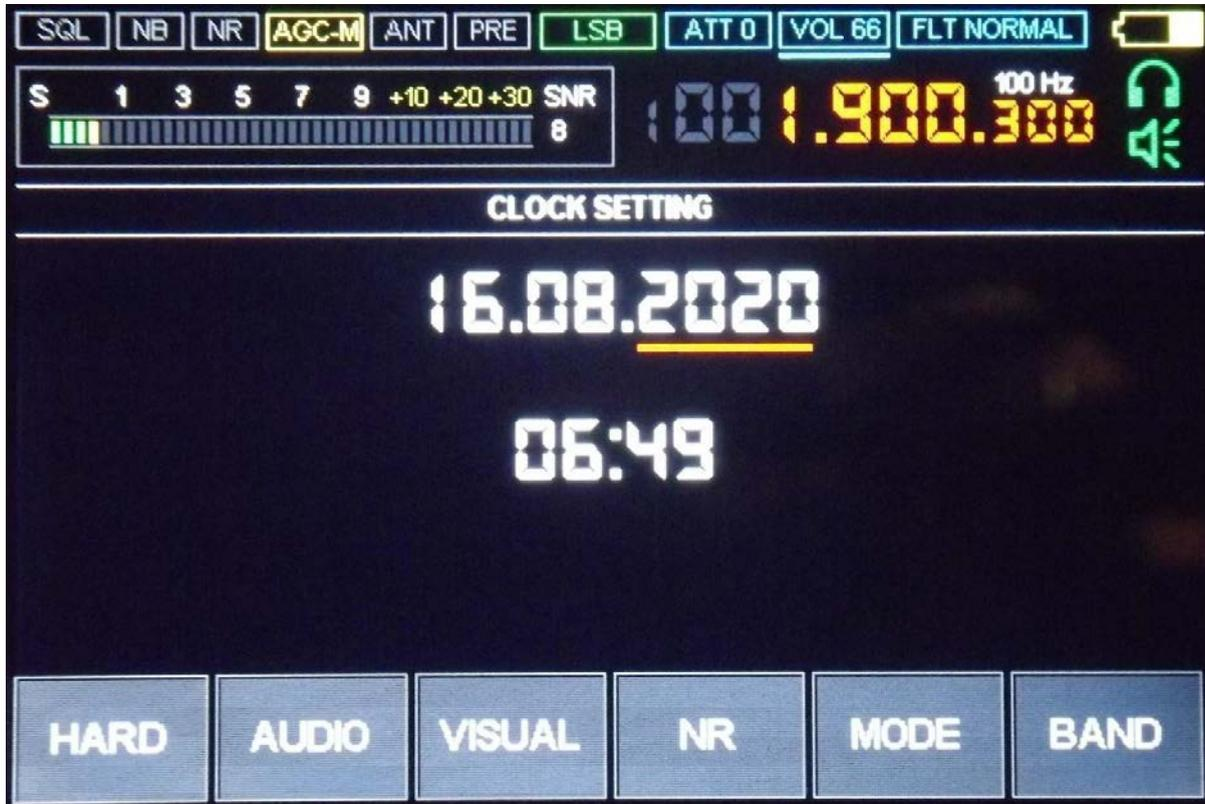
Clock setting menu is accessed by long pressing the RADIO (HARD) button. The setting is carried out using the ENC\_VOL encoder and its button. To save the value of the set time, you must press and hold the encoder button ENC\_VOL until the sound signal appears. The menu is exited by pressing the RADIO (HARD) button.
