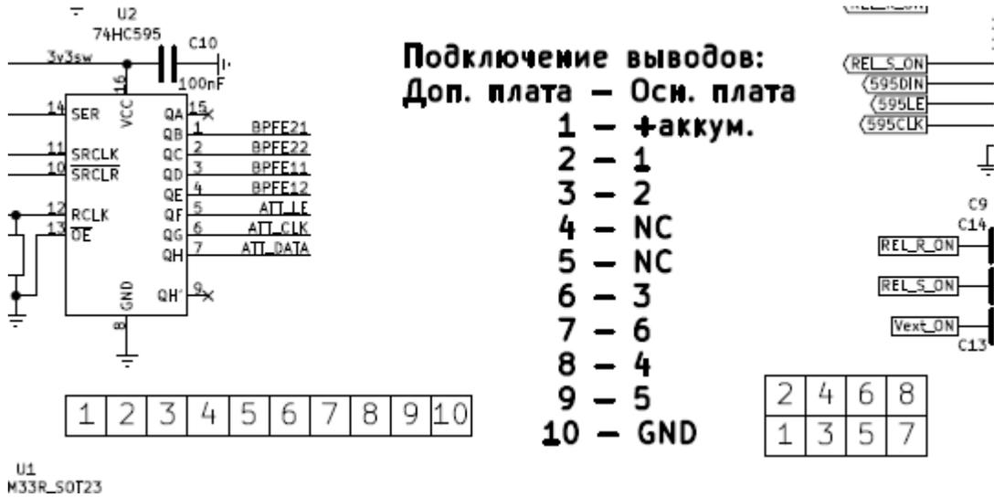
The location of the contacts is given in the form in which they are visible when mounting the board in the radio receiver:
