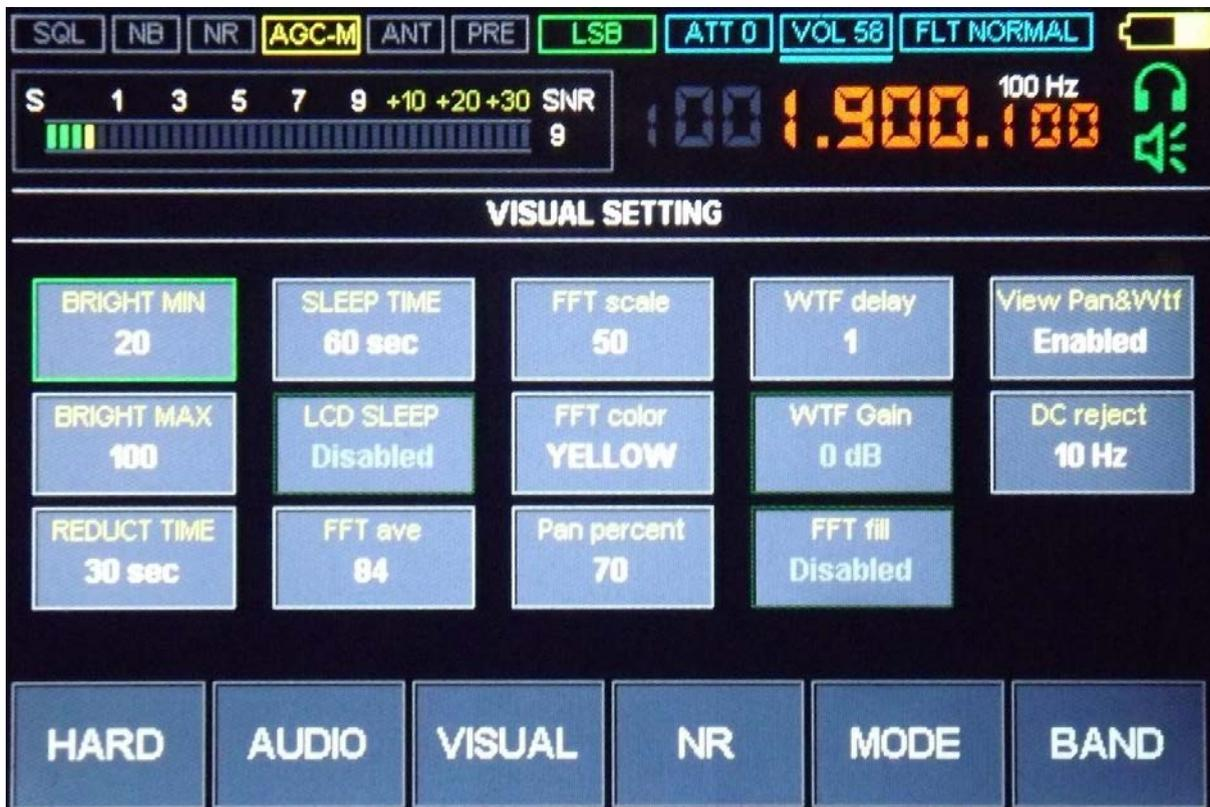
Entering the VISUAL menu is done by pressing the corresponding button. This menu contains various display settings for displaying information and display operation. Exit from the menu to the main screen of work is carried out by pressing the VISUAL button, or by pressing the ENC\_FREQ encoder button.
